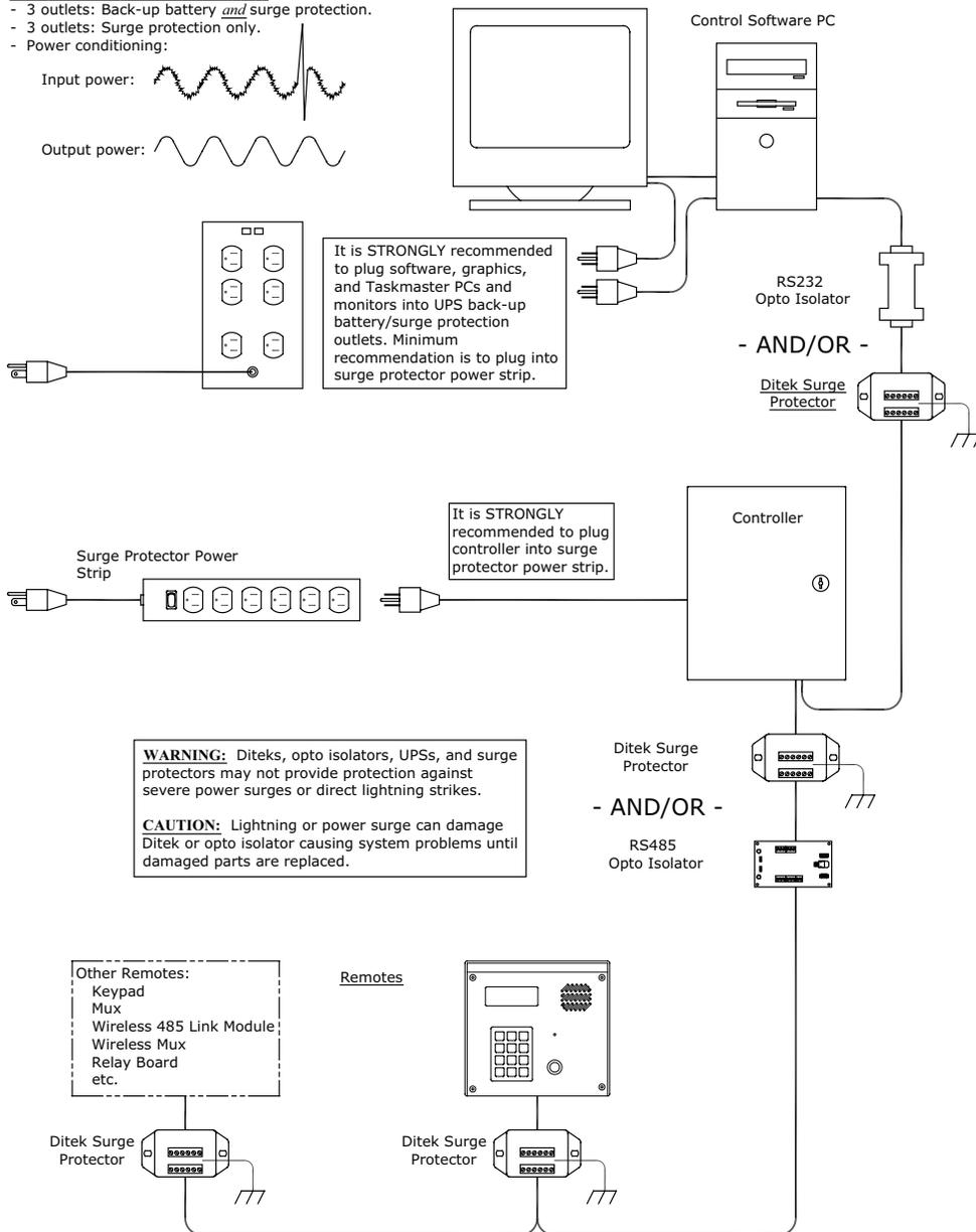
It is **STRONGLY** recommended to plug software, graphics, and Taskmaster PCs and monitors into UPS back-up battery/surge protection outlets. Minimum recommendation is to plug into surge protector power strip.
