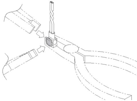
The crimping tool can be purchased from PTI Security Systems. For best results, crimp each connector three times in different places around the edge of the button. Verify that the button is evenly crimped all the way around and that it does not pop back up on one side.
