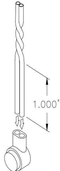
**NOTE:** Do not leave copper wire exposed. The outside sheathing is necessary for the strength of the connection.
