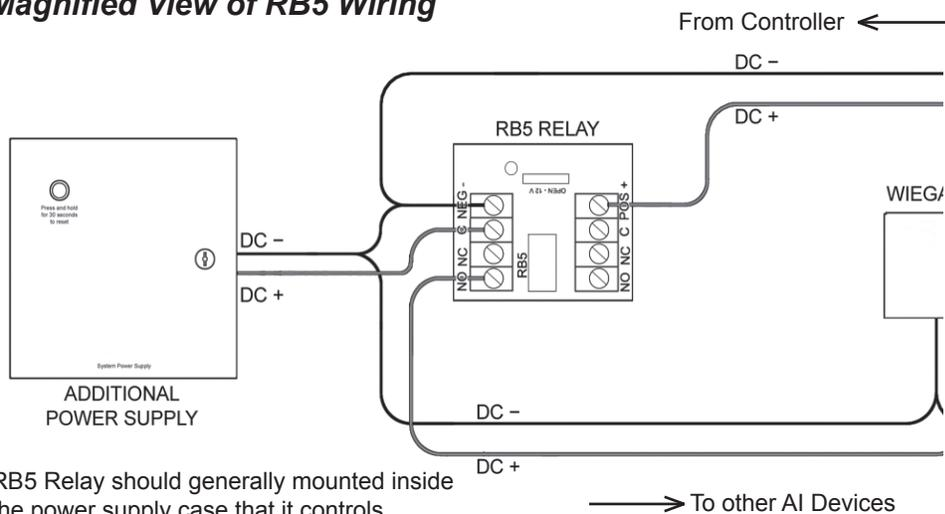
RB5 Relay should generally mounted inside the power supply case that it controls.
